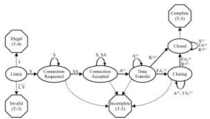
TCP session state machine. Dotted lines represent transition to a final session class. If a dotted line is unlabeled, the transition occurs after a specified interval of inactivity.
