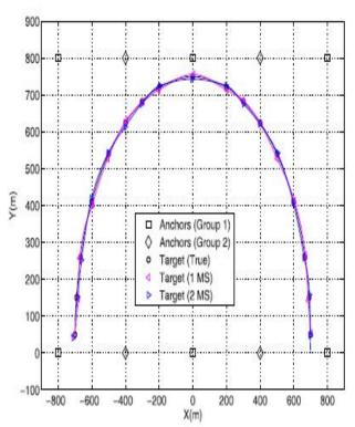
Fig 2: Comparision of tracking under different number of mobile sensors under circular trajectory.
