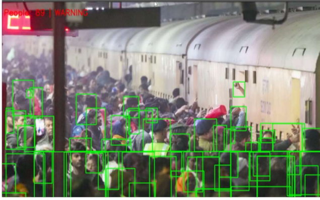
Fig. 9 Real-time crowd detection using YOLOv8m
