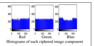
The histogram of each ciphered image component has tendency to be flat and so different of the original image
