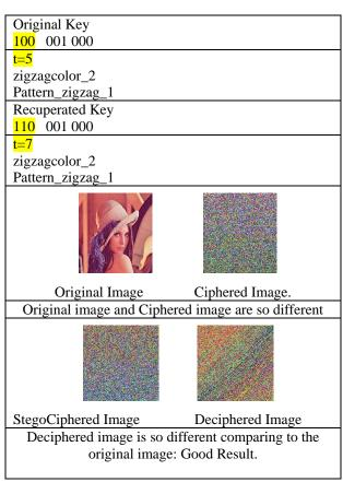
Figure 12:Original Key, Recuperated Key, Image obtained if the error is locating in repetitively order of the scrambling
