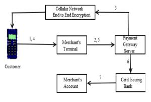
Fig. 3. Onsite Electronic Transaction
