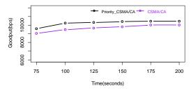
Fig 6: The Goodput comparison over varied times The 6% average performance is noted down against the standard protocol. It proves that the priority metric increases the delivery ratio to the greater extent and due to that the performance of the network is improved significantly.
