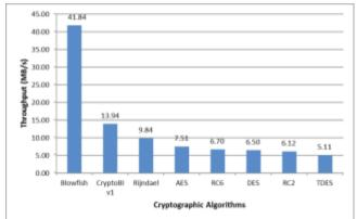
Figure 6: Throughput of each encryption algorithm (MB/Sec).
