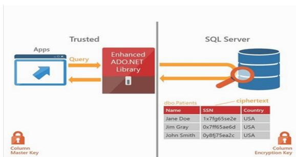
Fig 2: Always Encrypted Process [1]
