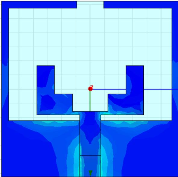
**Fig.9 H-field in the proposed UWB antenna**
