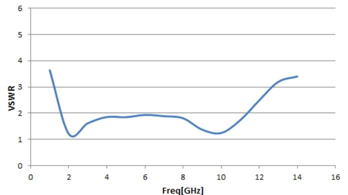
Fig.5. VSWR of proposed UWB antenna
