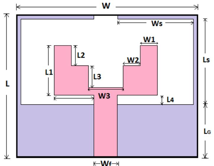
(b) Design parameters and dimensions of proposed antenna
