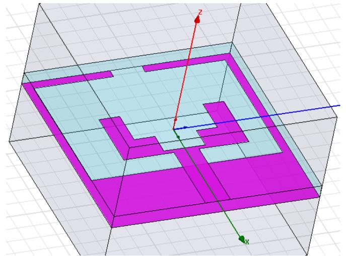
Fig.1. HFSS design of proposed antenna
