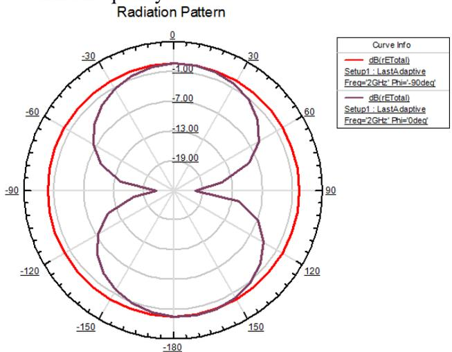
(a) Simulated Radiation pattern at 2 GHz
