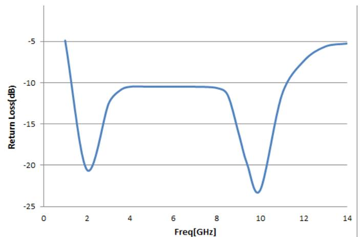
Fig.4. Return loss ( $S_{11}$ ) of proposed UWB antenna
