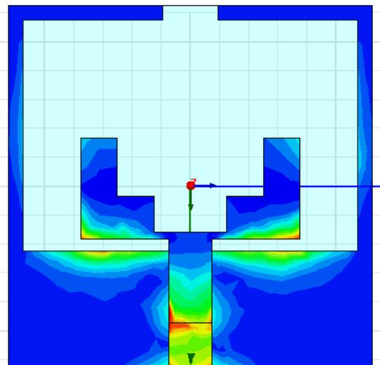
Fig.8 E-field in the proposed UWB antenna
